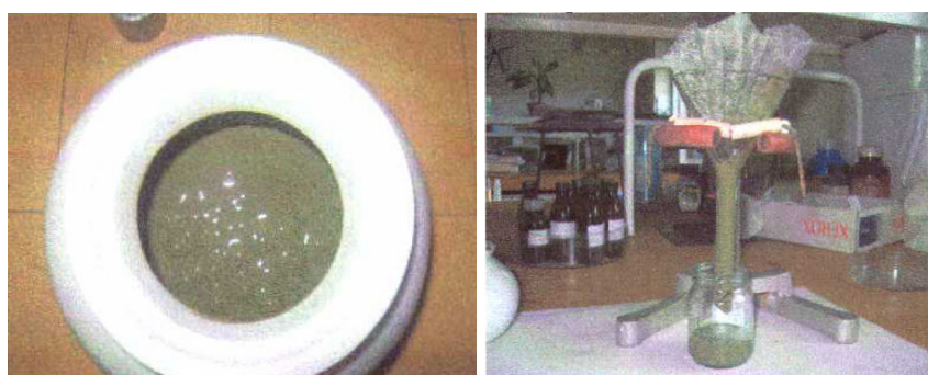
Figure no. 2. Wet grinding in a lab mill with porcelain balls and filtering the final product
