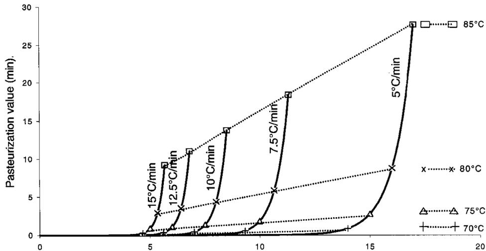
Figure 4. Pasteurization values during preparation as function of time cooking for five rates of growth temperature (15.0, 12.5, 10.0, 7.5 and  $5.0^{\circ}\text{C}/\text{min}$ ) and four finally temperature ( $70$ ,  $75$ ,  $80$  and  $85^{\circ}\text{C}$ ).  $D_{70} = 2.95$  min and  $Z=10^{\circ}\text{C}$ .
