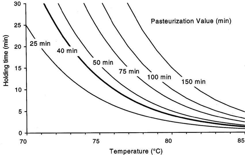
Figure 5. Curves of pasteurization for different temperatures between 70-85<sup>0</sup>C as a function of time of storage
