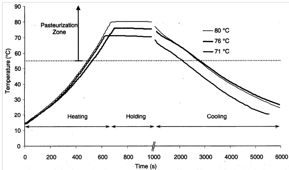
Figure 2. Temperature profile inside sample set for three points (71, 76 and 81°C)
